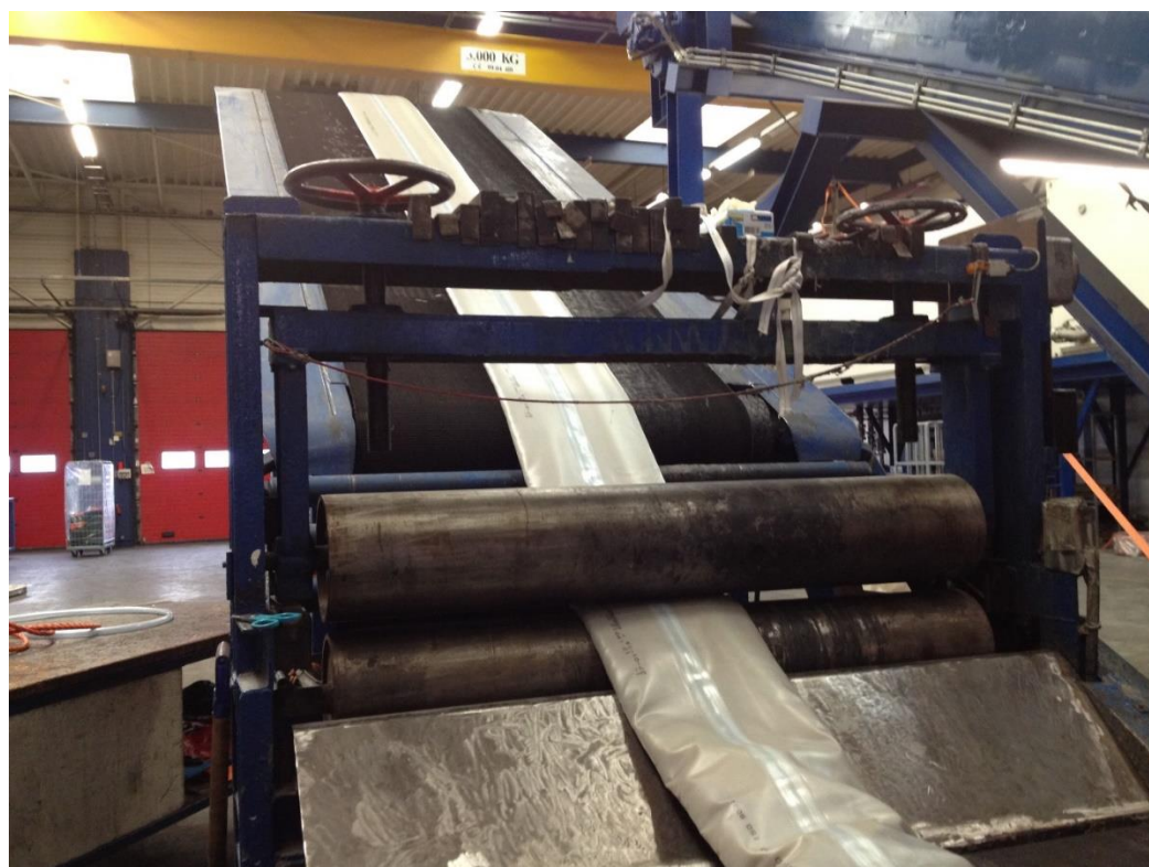
Figure 1 Impregnating a liner with resin.
